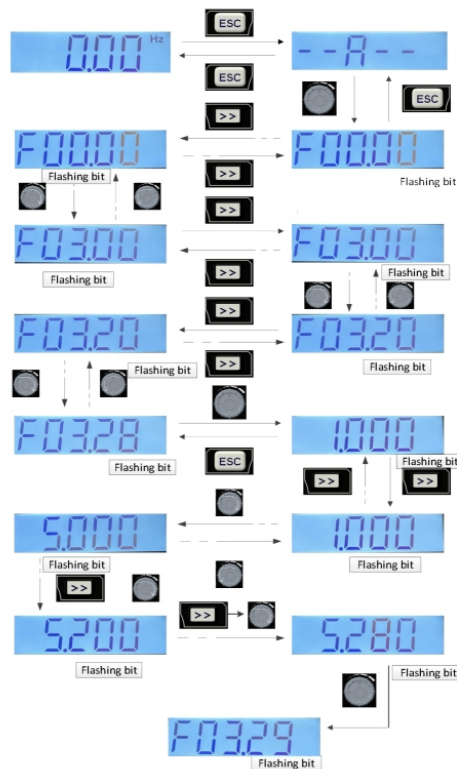
Fig. 4-3 Flowchart from Power-on to F03.28=5.28 Setting
